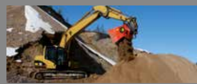
ALLU Screener Crusher Screening, crushing, mixing, aerating, and loading in one step operation
